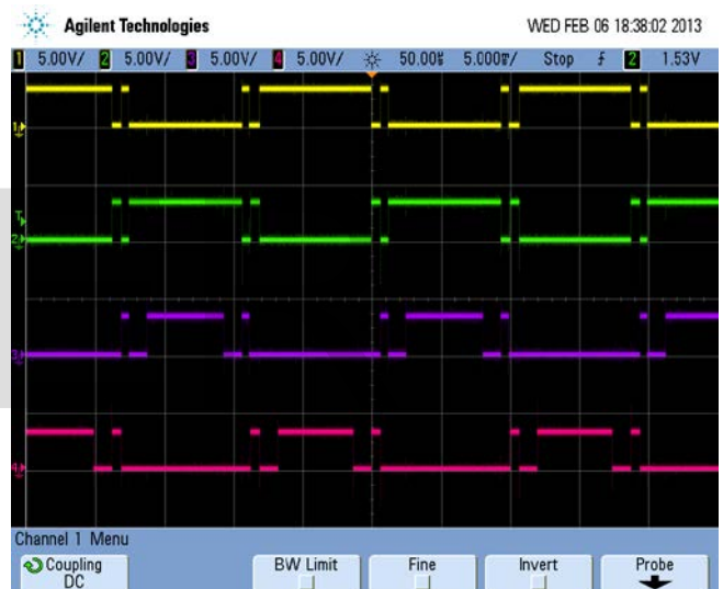
Fig 5. PWM pulses to the Inverter switches S6, S7, S8,S9
